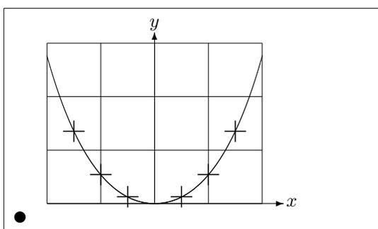
In this figure, each symmetric half of the catenary  $y = \cosh x - 1$  is approximated by a quadratic Bézier curve. The right half of the curve ends in the point  $(2, 2.7622)$ , the slope there having the value  $m = 3.6269$ . Using again equation (5.1), we can calculate the intermediate control points. They turn out to be  $(1.2384, 0)$  and  $(-1.2384, 0)$ . The crosses indicate points of the *real* catenary. The error is barely noticeable, being less than one percent.
